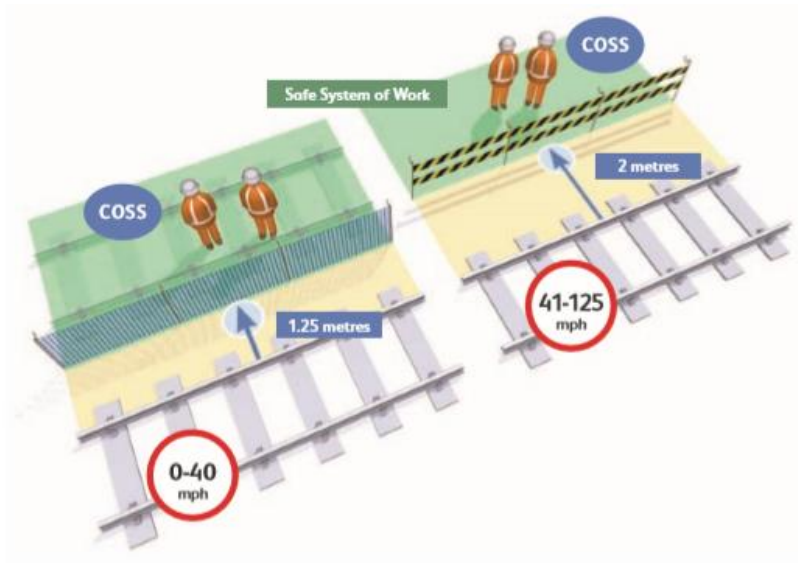
Examples of fenced Safe System of Work – (left) using plastic netting on a blocked line and (right) using barricade tape in the cess.
